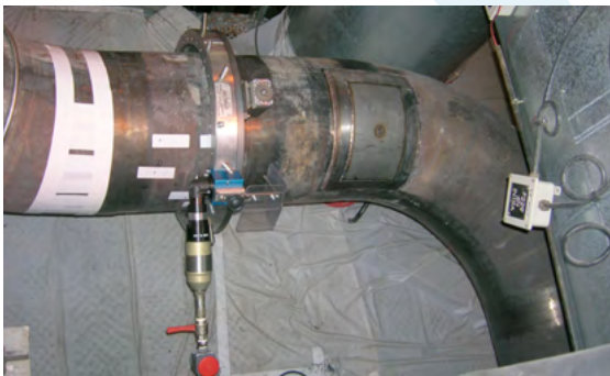
TTLW610 Tube Cutting & Beveling equipment with pneumatic drive
